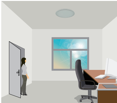
With sufficient natural light, the light does not switch on when presence is detected.
